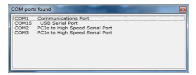
**Double click** on an entry to make it the current COM port. If already connected you must disconnect and then connect to open the newly selected COM port.
