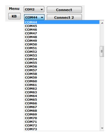
Selects the serial port used to communicate with other software such as the ASCOM Focuser Driver AGF\_AP\_LX200 Virtual absolute focuser driver or MegaStar.
