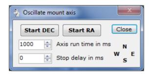
Runs the RA and DEC servo motors in forward then reverse direction with a delay between switching directions.
