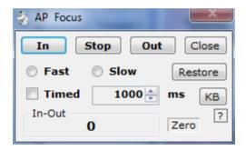
Controls a focus motor connected to the **FOCUS** connector on the GTO Servo Controller. Must be a 12VDC motor. The Meade 1201 Microfoucser will only work on a CP3 controller using Fast.
