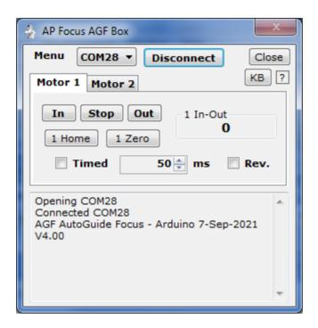
Controls focus motors connected to the AGF FOCUS Controller Box. Must be a 12VDC motor
