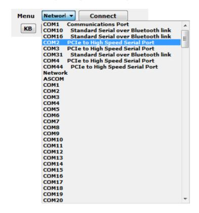
Selects the serial port used to communicate with the mount's GTO Servo Controller.
