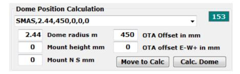
The geometry of the dome and telescope location on the mount are entered here and used in the **Calc. Az** function to determine the azimuth of the dome opening for a given dome and telescope combination.
