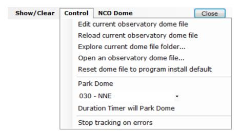
Observatory domes file management. Defines dome and telescope combinations for setting different configurations.
